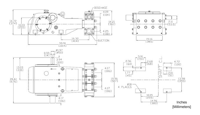
Power Required:  $HP = \frac{GPM \times PSI}{1450}$
